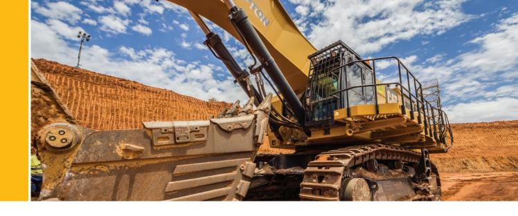
Analysis of the results showed the Cat 6015B was clearly more fuel efficient and productive. The 6015B took just 6.8 cycles to load a truck compared to the Hitachi's 8.8, and it took just 2.29 minutes to load each truck compared to 3.16 minutes for the Hitachi. When excess waiting time was factored out for both shovels, the Cat 6015B loaded 1704 tonnes per hour — an impressive 28 percent more than the Hitachi's 1323 tonnes per hour.
