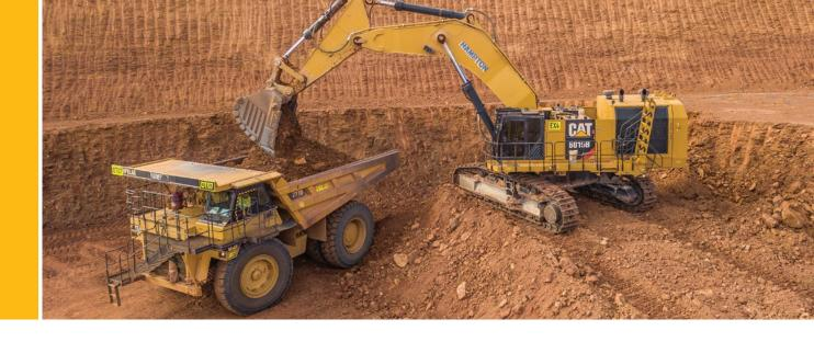
Weighing in at 140 tonnes and with an 8.1 cubic metre bucket, the Cat 6015B fills a long-standing gap in the Australian hydraulic excavator market. But how does it stack up against its rivals?
